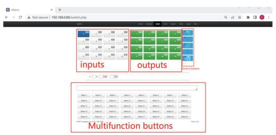
All input and output ports can be renamed, Multi-function buttons area, through simple Settings, can be controlled through the serial port peripheral devices, such as projector switch. No setting is the scene call shortcut button.
